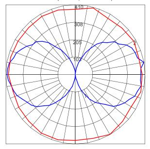
Maximum Candela = 410.2; Located at Horizontal Angle = 300; Vertical Angle =100 #1 - Vertical Plane Through Horizontal Angles (300 - 120) (Through Max. Cd.) #2 - Horizontal Cone Through Vertical Angle (100) (Through Max Cd.)
