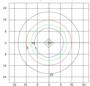
Isofootcandle Plot shows light distribution pattern at ground level with custom LED light engine with no shield. Readings have been taken assuming the photometric center of the luminaire to be 8.93 feet above ground level. IES files for standard lamps are available on our website.
